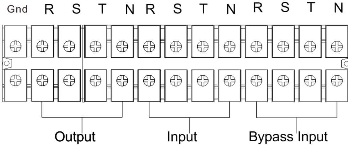
**HV 30K(L)/40K(L)双输入端子排示意图**
