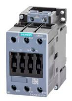
Contactor AC 220V 50/60 HZ AC3 18,5 kW 400 V 3 pole, mod. S2 screw terminal
